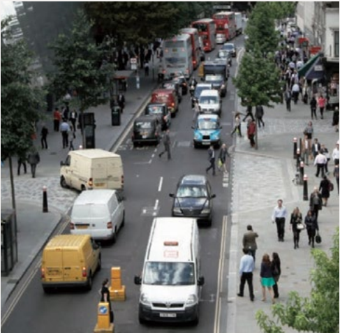
Footway widening with raised loading pads and greening create a more enjoyable environment for walking in the City of London. Credit: City of London
