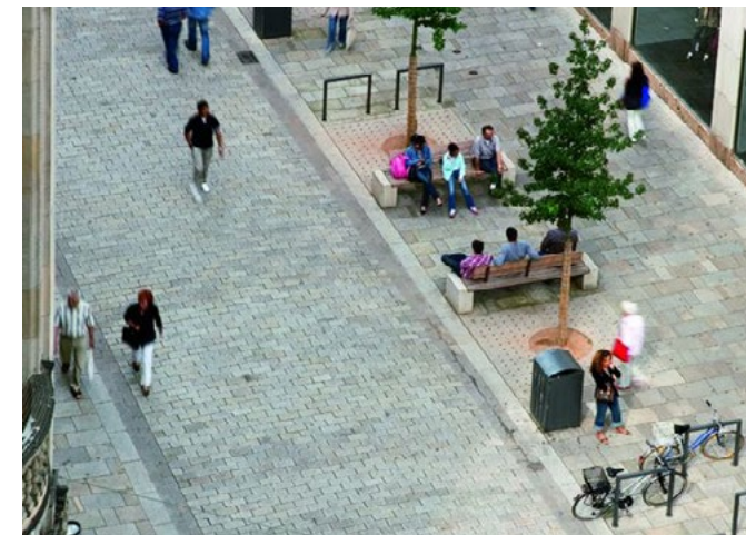
Raised carriageway bordered by seating, trees and cycle parking in Wiesbaden, Germany. Credit: Strauma
